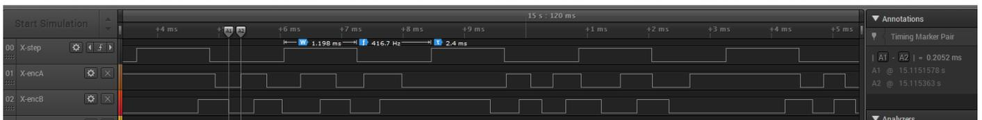
When running at 500 steps/s the operation is noticeably smoother. The above shows a frequency of 416.7Hz, this is partly due to the granularity of the stepper frequency generation (which is poor, should be using DDS), and partly due to the ISR missing interrupts due to controlling 2 or 3 steppers simultaneously.
