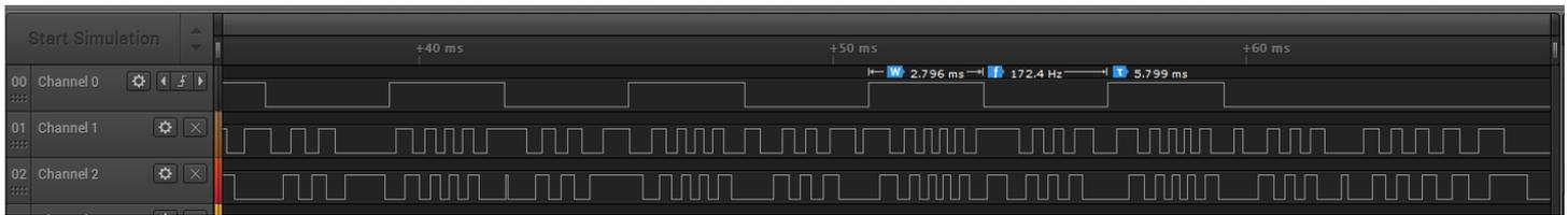
The above capture shows the software 'stopping' the step pulses during deceleration. The frequency should slow down to 50Hz, but here it's still 170Hz and just stops. There is nothing in the encoder waveform to suggest any problem, other than the previously mentioned forward/reverse counts (but all valid waveforms). The very short pulse on 'Channel 2' (X-encB) about 8 pulses in is about 50us, and is perfectly valid.
